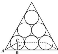
In the figure,  $CA = 2r$ ;  $AB = r\sqrt{3}$ . The base of the triangular package is  $4r + 2r\sqrt{3}$ . Since the triangle is equilateral, its area is
